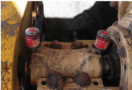
Labyrinth seal purging on a small slurry pump
